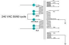
For Japan 100 volt connect 1 to 4 and 2 to 5 Use 1,4 and 2,5 for line connection.
