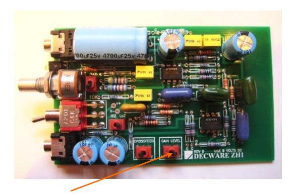
It is located here and is best adjusted during a serious listening session because what it does is subtle. The ZH-1 has two stages of gain, hence to Burr Brown Operational amplifiers. This switch adjusts the amount of dynamics that are allowed from the first stage to the second. Usually the best approach is to set this switch to "HIGH" if the Impedance switch is set to 32K or to "LOW" if set to 10K.
