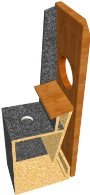
The final modifications included sealing the bottom of the main cavity and putting a round 3/4" long port at the top of the cavity to set the low frequency cut off point.
