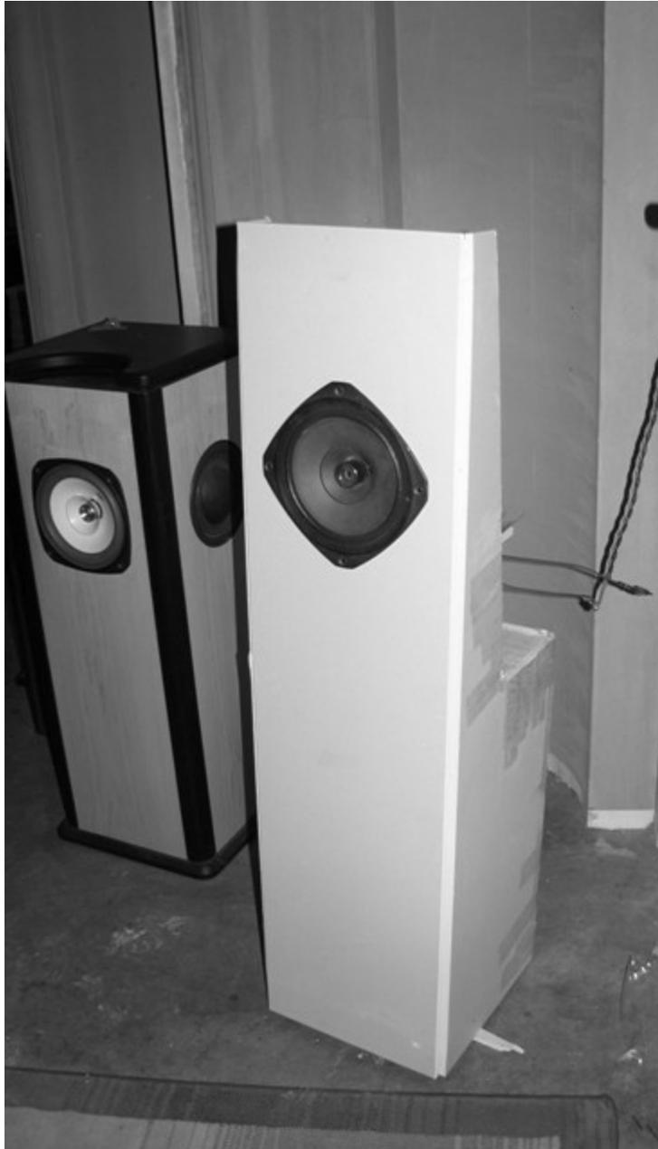
Here is a view of the drywall prototype with a modified FE206E installed.
