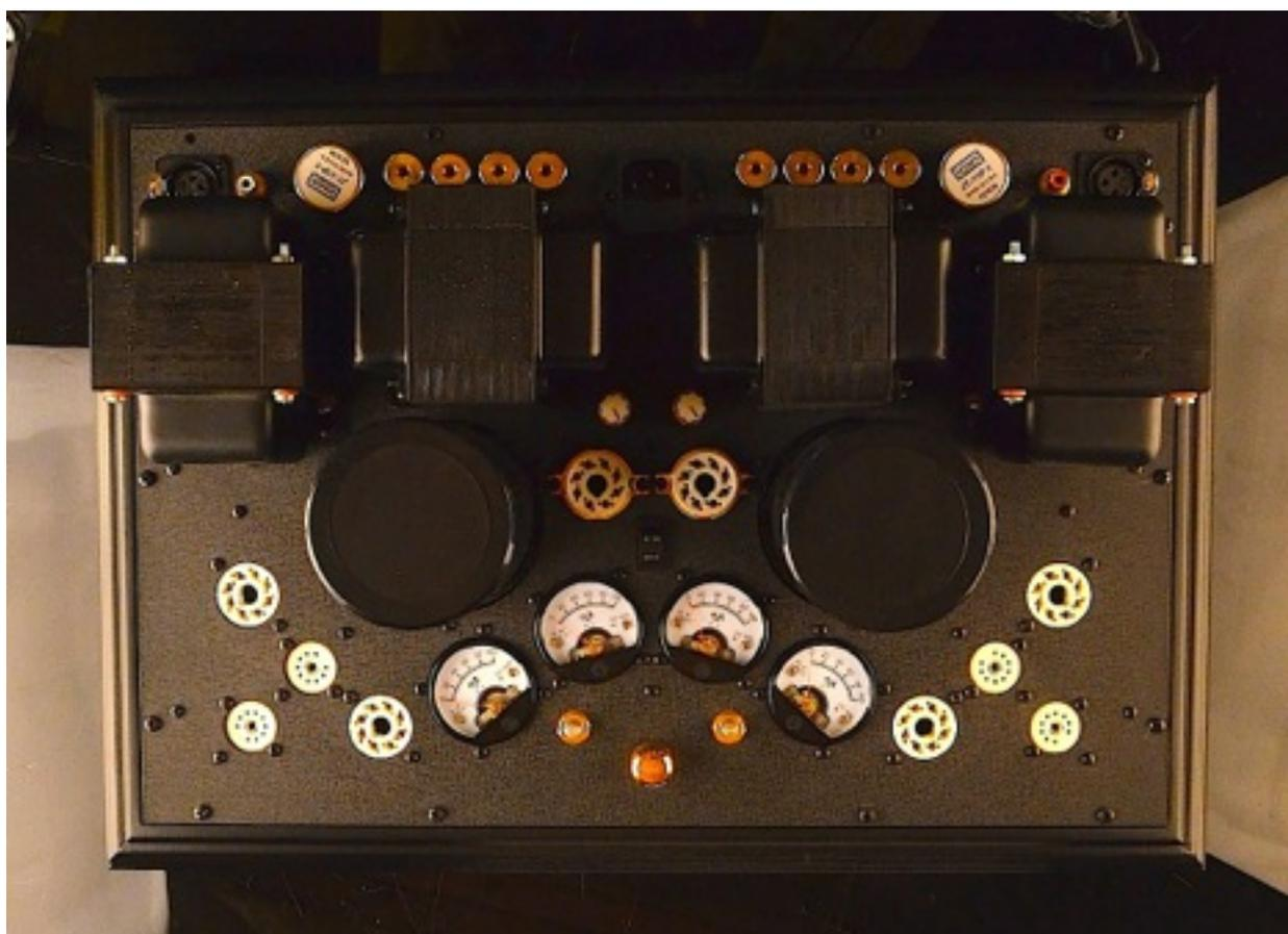
The important thing to notice about your amplifier is that it is actually TWO mono amplifiers that are laid out symmetrically in a mirror image pattern from an imaginary centerline between the IEC plug for the power cord and the volume control. In other words, everything on the left side of the amp is repeated in a mirror image on the right side of the amp. From this view, the left side of the amp is typically used for the left channel and the right side, the right channel.
