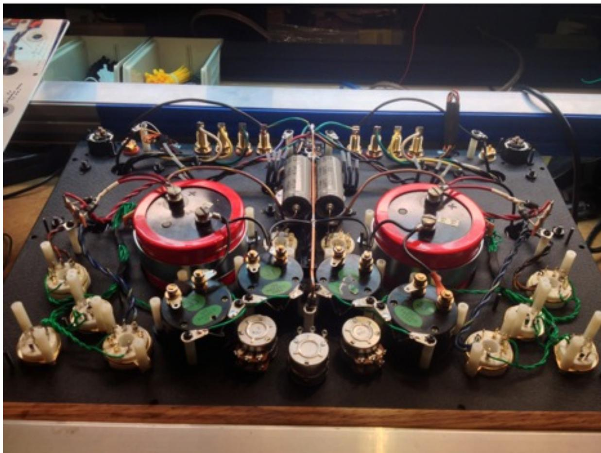
Shown above is a Zen Mystery Amp ready for its final soldering phase. What you see completed in the picture is only the power supply. It is now ready for the hand full of parts that make up the audio circuit.
