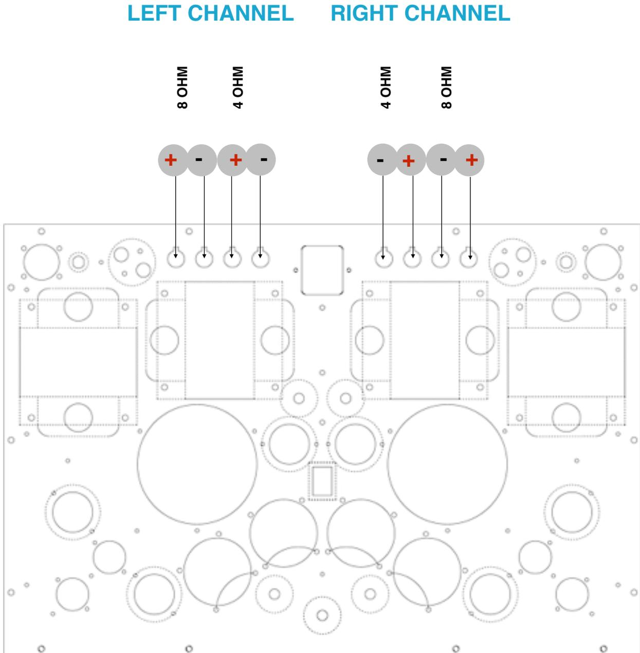
As you can see, there is a separate positive and negative post for both 4 ohm and 8 ohm speakers. Use only one pair at a time.
