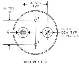
USE ONLY #4 TYPE B SELF TAPPING SCREWS IN HOLES "M". ALLOW NO MORE THAN 0.15" PENETRATION INTO TRANSFORMER HOUSING.
