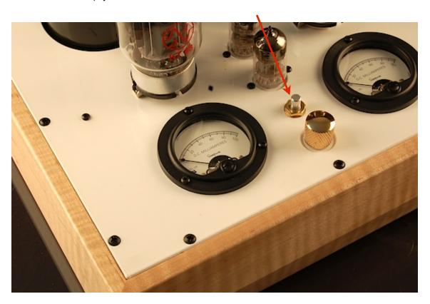
In the picture above you can see the meter on the left is for the KT88 output tube directly behind it. Same for the meter on the right. These meters show how many milliamps of current are going through each output tube. Since this is a push pull amplifier, the objective is to get both tubes to draw the same amount of current so that they match. This gives the best performance and the most power.
