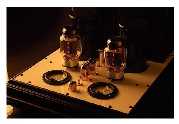
1 Channel 60 watt Vacuum Tube Amplifier
