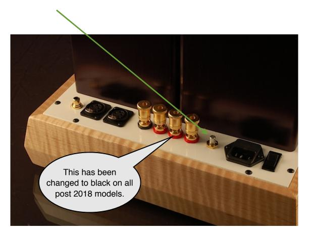
The range of this control varies with output tubes. The ideal operating point for KT88's in this amplifier would be between 60 and 70 milliamps. 80 milliamps should be considered the absolute maximum. Running any higher will sacrifice headroom and create more heat.
