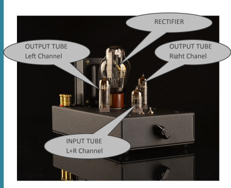
Tubes should be carefully installed prior to hooking up your product.
