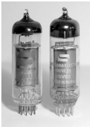
The tube on the left is an acceptable SV83 output tube for use in this amplifier. The tube on the right with the smaller logo is NOT acceptable for use in this amplifier or any Decware amplifier.
