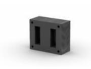
Our transformers cores (shown left) are made with M-6 29 Gauge - 0.014" (0.355 mm) Grain Orientated Electrical Transformer Steel Lamination with steam blue oxide on the surfaces and edges to minimize stray losses between laminations.
