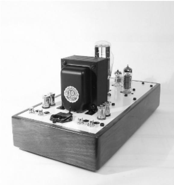
With the jacks vertically mounted at the rear of the amplifier, it is possible to push the amp all the way to the rear of a shelf. **However, we recommend keeping a 2 inch spacing on all sides and at least 6 to 10 inches of space above the amplifier.**
