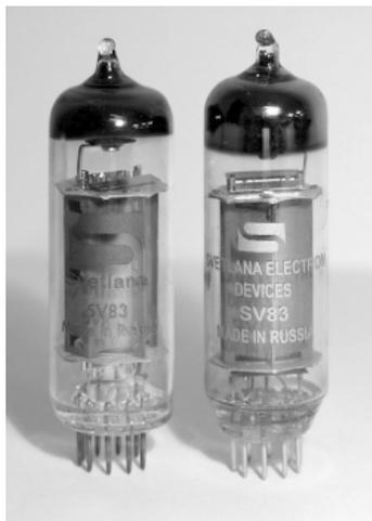
The tube on the left is an acceptable SV83 output tube for use in this amplifier. The tube on the right with the smaller logo is NOT acceptable for use in this amplifier.
