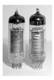
The tube on the left is an acceptable SV83 output tube for use in this amplifier. The tube on the right with the smaller logo is NOT acceptable for use in this amplifier or any Decware amplifier.
