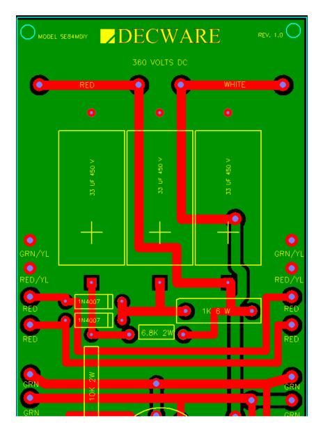
The silk screen is printed on the bottom side of the board. The tube sockets mount to the top side of the board only. Parts can placed on either side of the board depending on how the board is mounted:
