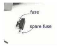
The fuse is a 3 amp, 20mm glass fuse. You can use fast or slow blow type replacements in the amp. It is located INSIDE the IEC connector. To access it, remove the power cord and take a small screwdriver to pry the little door open. It will come completely out of the IEC connector and not only holds the fuse, but has a spare fuse in it as well.
