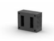
Our transformers cores (shown left) are made with M-6 29 Gauge - 0.014" (0.355 mm) Grain Orientated Electrical Transformer Steel Lamination with steam blue oxide on the surfaces and edges to minimize stray losses between laminations.
