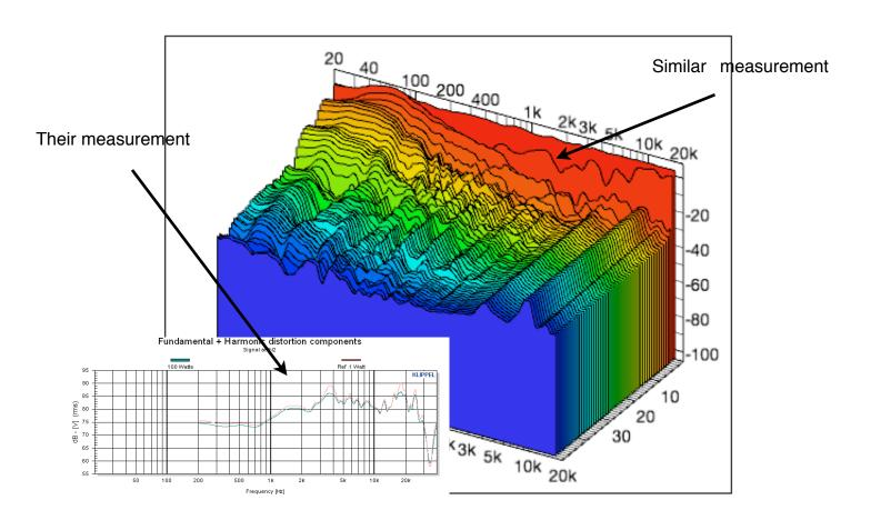
It then became obvious that there was a 1ms delay in the measurement software causing it to read the response just before the stimulus signal. Even though I thought it was awfully good response, I also knew the measurement system was working because of the waterfall plots and a myriad of other reasons. And what I was hearing was unusually smooth which helped to confirm it. So I guess the joke was on me.
