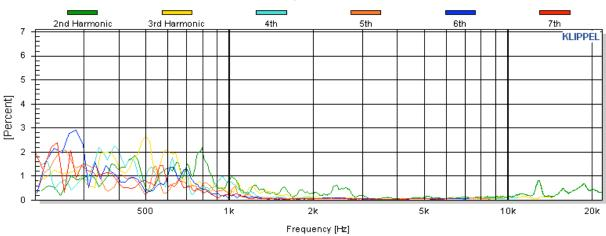
Harmonic distortion is from 200 cycles to 20,000 cycles.
