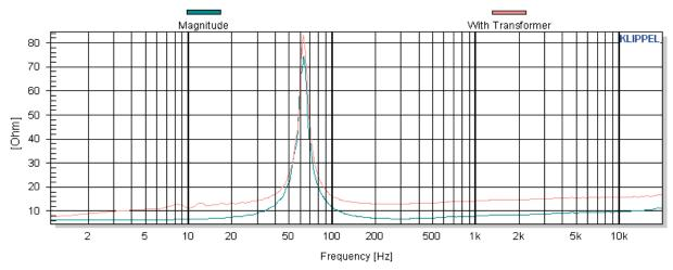
Note that the graph above is the impedance of the FRX driver with and without it's magnetic coupling transformer.
