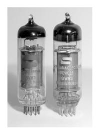
The tube on the left is an acceptable SV83 output tube for use in this amplifier. The tube on the right with the smaller logo is NOT acceptable for use in this amplifier.
