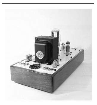
With the jacks vertically mounted at the rear of the amplifier, it is possible to push the amp all the way to the rear of a shelf. **However, we recommend keeping a 2 inch spacing on all sides and at least 6 to 10 inches of space above the amplifier.** Avoid closed cabinets. The better the ventilation around your amplifier the cooler it will run.
