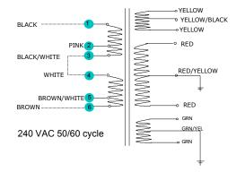
NOTE: We recommend wiring the primary for 240 volts even if your voltage is 220 or 230. Use a 3 amp fuse. NOTE: The BLUE wire (not shown) is a bias tap and is NOT USED in this circuit.
